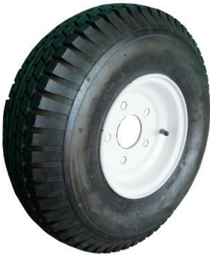
Photo Below: TWA0253 – 5.00 x 8 – 8 ply highway tyre fitted to a 3.75 x 8 five hole wheel. P.C.D. = 114.3mm (Ford)
