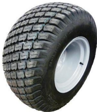
Photo Below: TWA0051 26/12.00 x 12 – 6 ply Turf Tyre fitted to a 10.00 x 12 wheel with 5/114.3 PCD (Ford)
