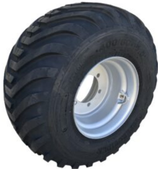
TWA0017 – 12.5/80-18 R4 Lug tyre fitted to a 18 x 9 six hole wheel.
